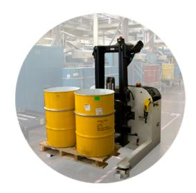
AGVs navigate using laser beams. Their laser navigation is extremely accurate, so much so, that they are wearing tracks in the factory's wooden floor after taking exactly the same path every single time they travel!
