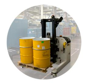
AGVs navigate using laser beams. Their laser navigation is extremely accurate, so much so, that they are wearing tracks in the factory's wooden floor after taking exactly the same path every single time they travel!
